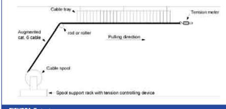
cable, the larger the minimum bend radius. In other words, if a minimum bend radius under load does not impact the performance of the larger category 6A cable, it will not impact smaller diameter cables such as category 5e and category 6 UTP.
