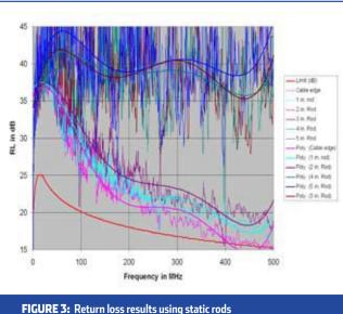
\*Note: The polynomial curve provides a trendline for analyzing this fluctuating large data set.
